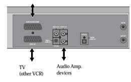
To copy to your player from another video machine, connect the two machines with a cable between their EURO AV (SCART) sockets and select as programme "AV 1/AV 2" or "F. AV" (front sockets) using the [AV]. [PR+/-] or [0, 0]button.
